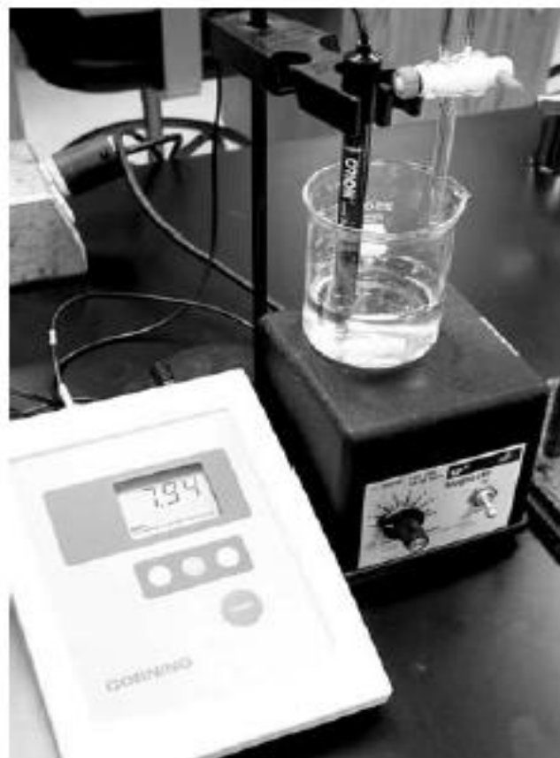
FIGURE 14.11 A setup for a potentiometric titration.
